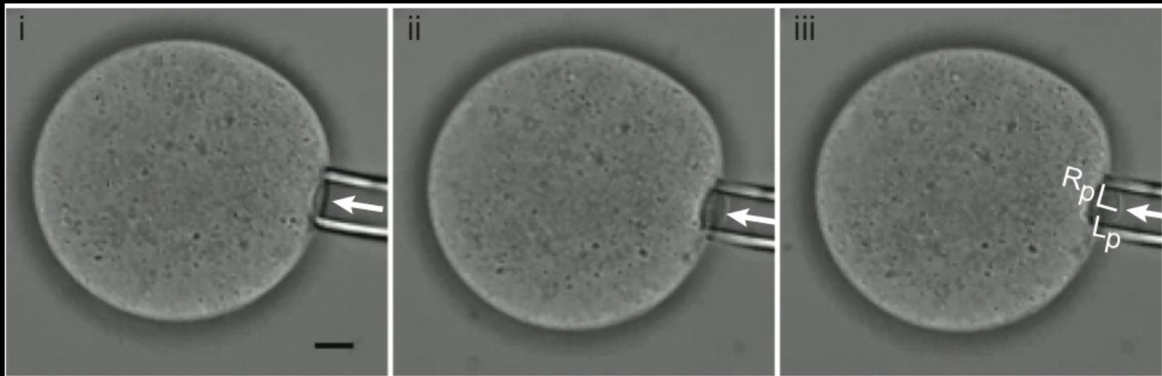
$$T_{\text{eff}} = \text{Aspiration pressure} / (2 \times (1/\text{pipet radius} - 1/\text{cell radius}))$$
