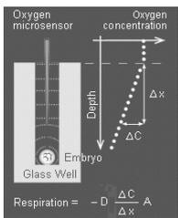
The oocyte/embryo at the bottom of the well uses O<sub>2</sub>, a diffusion gradient is established down the length of the well.
